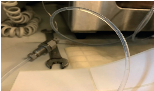
Figure S8. Photograph of the obtained slug-flow of the aqueous phase (small bubbles) and the MTHF organic phase (larger slugs).
